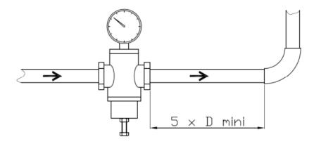
**Upstream shut-off:** Please provide for aisolating valve upstream the 681 valve, because it is not necessarily watertight at zero flow condition and do not constitute a shut-off device.
