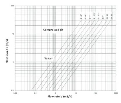
For water or similar liquids, do not exceed a 2 m/s flow speed. For compressed air, choose a flow speed between 10 and 20 m/s.
