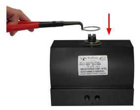
B10. Place the washer over the top of the driveshaft. Place and fasten the upper Circip around the top of the driveshaft by using external drop nose Circlip pliers.
