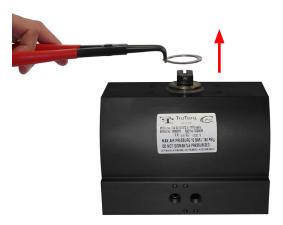
A7. Remove the Circlip at the top of the driveshaft by using external drop nose Circlip pliers. Then remove the washer.
