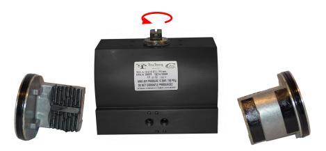
A6. Remove the pistons out of the body by turning the top of the shaft, anti-clockwise\*, by using an appropriate tool
