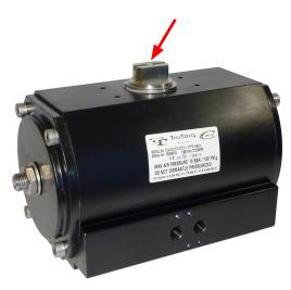
A1. Check/note the shaft position, when the actuator is in a unpressurized state, in relation to the actuator before the dismantling. The intention is to ensure that the actuator has the same function after reassembly (Fail Closed, Fail Open or Crossmount).
