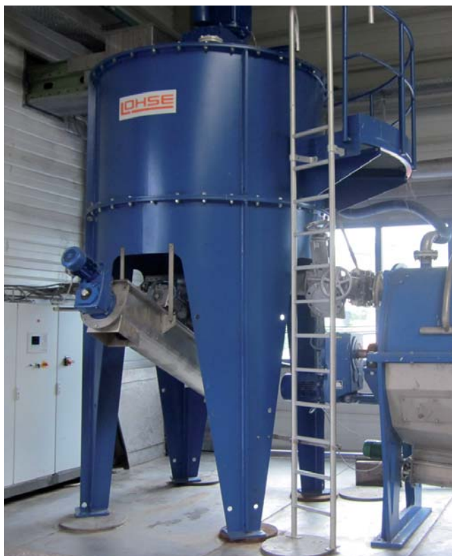
LMC4 + LMC6 with base of steel construction
